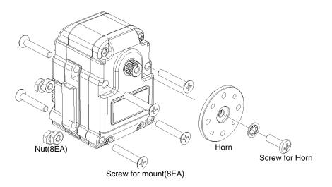
The 8 sets of Nuts & Screws are only used when a Dynamixel is mounted to other equipment.
